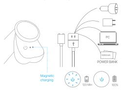
It is recommended to use the charging cable with a 5V/1A charger to avoid damage caused by improper charging.
